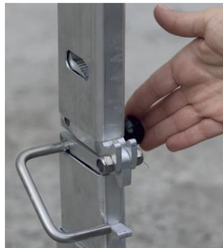
Press the bracket against the spring.
